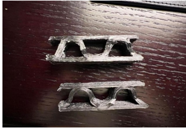
Figure 8. The sandwich's physical piece after the compression test
