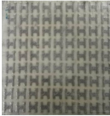
Figure 11. Photograph of laminated composite containing conductive fiber FSS material
