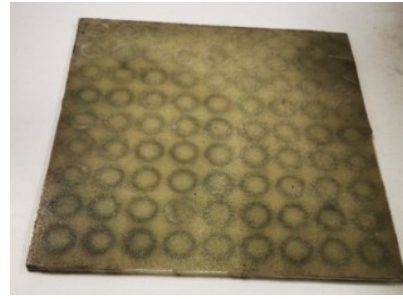
(b) Laminated composite containing conductive fiber FSS material
