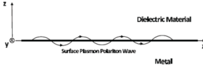
Figure 1. Surface Plasmon Polariton wave model
