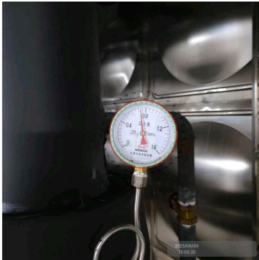
Figure 2. A Result of gauge detection and scale calibration. The circular dial is correctly identified with scale lines marked at 10-degree intervals, and numerical values are annotated around the dial for reference
