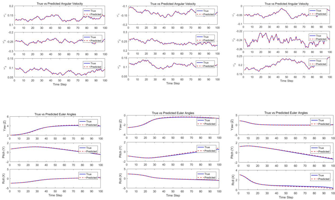
Figure 4. Prediction results of angular velocity and Euler angles for three representative test trajectories using the Koopman-based model
