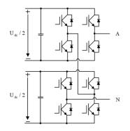
Figure 3. Single-phase cascaded three-level inverter topology [1]
