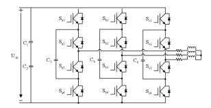
Figure 2. Topology of FC three-level inverter [1]
