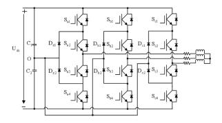
Figure 1. NPC three-level inverter topology [1]
