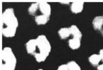
Figure 7. Images of benzene molecules were obtained using a scanning tunneling microscope
