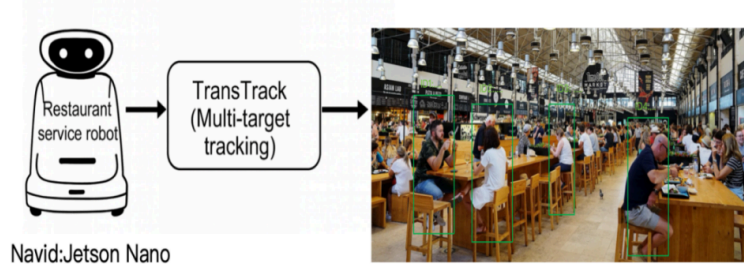
Figure 3. TransTrack integrated into the vision pipeline of an indoor restaurant service robot
