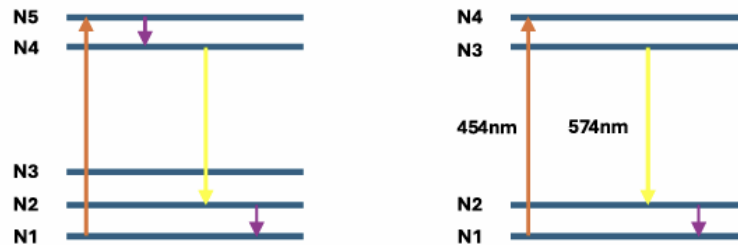
Figure 1. Simplification process of \text{Dy}^{3+} energy level diagram in the 560-600nm band
