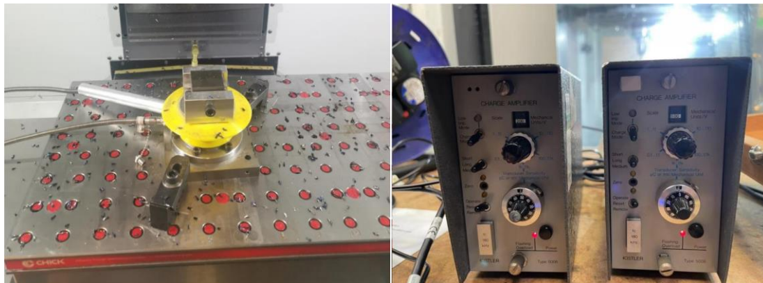
Figure 2. Kistler's dynamometer with mould (left) and charge amplifier (right).
