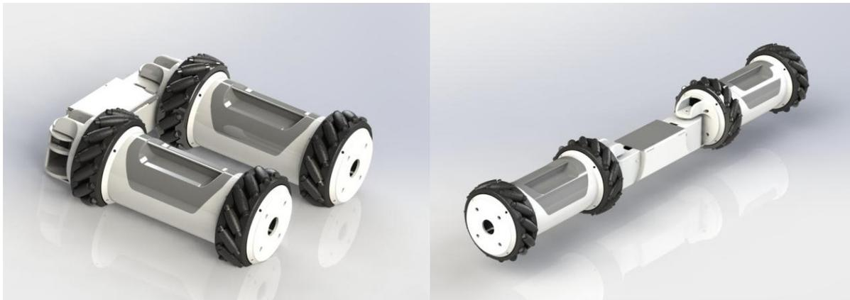
**Figure 1.** Rendering of 3D modeling. A: Rendering of the Deformable Smart Car in “U” shape; B: Rendering of the Deformable Smart Car in “I” shape.
