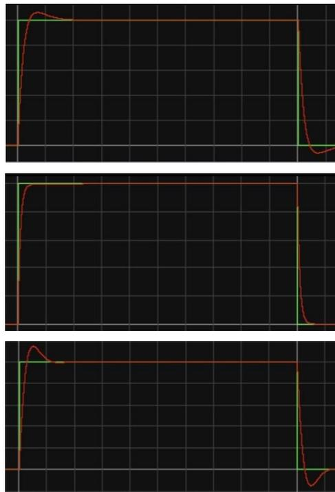
**Figure 7.** Reference tracking for different value of  $K_p$  and  $K_i$  in Falstad. A: Reference tracking for  $K_p=1$ ,  $K_i=20$ ; B: Reference tracking for  $K_p=2$ ,  $K_i=20$ ; C: Reference tracking for  $K_p=1$ ,  $K_i=40$ .
