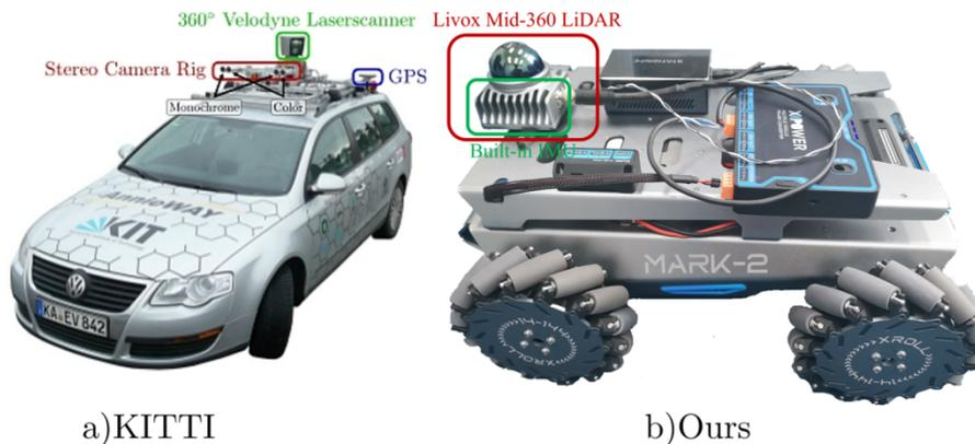
**Figure 4.** Recording platform with sensors (a) from KITTI dataset [20] and (b) our private dataset
