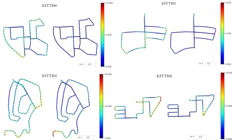
**Figure 8.** Trajectories (left) generated by VoxelMap compared to trajectories (right) after correction by our approach. The color bar on the right indicates distance error between the generated trajectory and the ground truth. Unit: m
