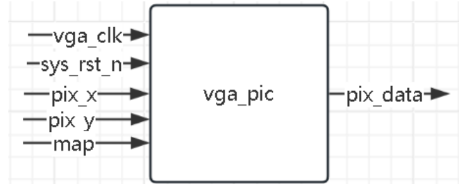
Figure 4. Block diagram of VGA image data generation module.
