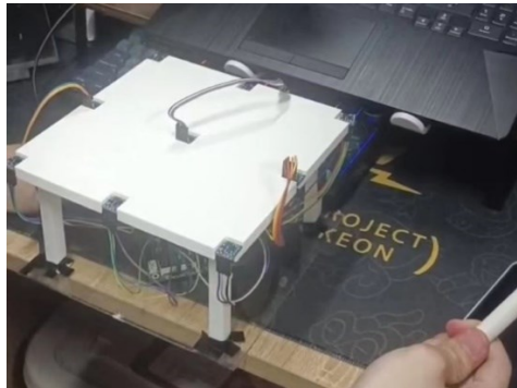
Figure 4. photograph of magnetic sensor arrays and pen
