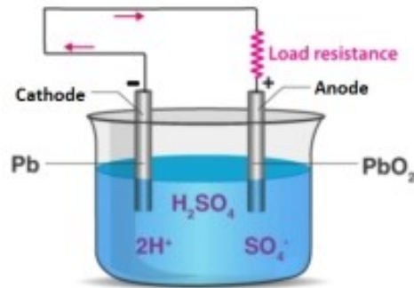
Figure 1. Lead-acid battery discharging.
