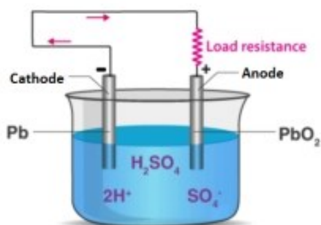
Figure 1. Lead-acid battery discharging.
