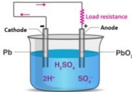
Figure 1. Lead-acid battery discharging.
