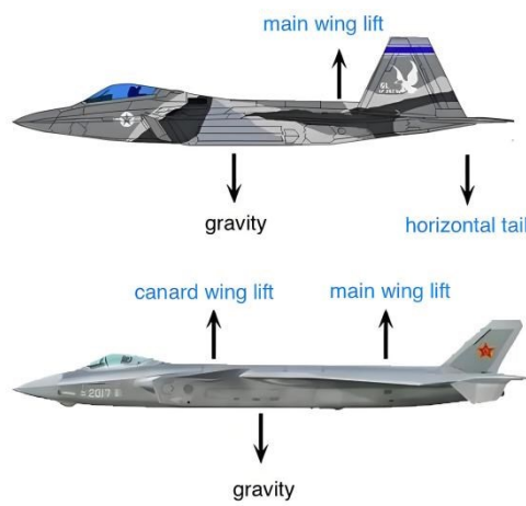
Figure 3. Schematic diagram of lift for conventional and canard layout aircraft
