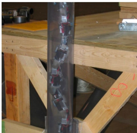
Figure 1: View of a snake robot climbing the inside of a pipe [1]
