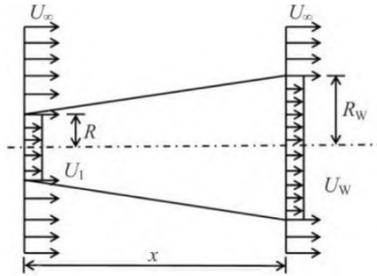
Figure 1: Wake Effect Cross-Section in Wind Turbine Arrangement[5]
