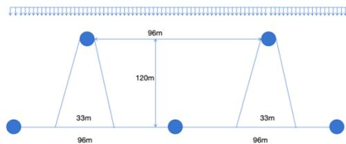
Figure 3: Centralized Wind Turbine Arrangement Plan
