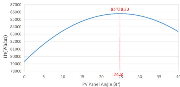
Figure 2: Relationship Between Photovoltaic Panel Inclination Angle and Annual Solar Radiation
