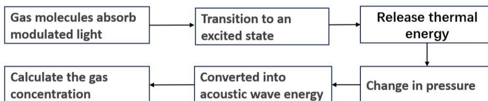
Figure 1: Schematic diagram of the principle of photoacoustic spectroscopy technology
