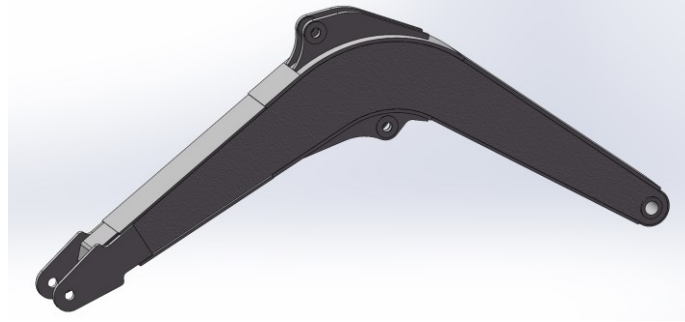
Figure 1: Three dimensional diagram of excavator boom
