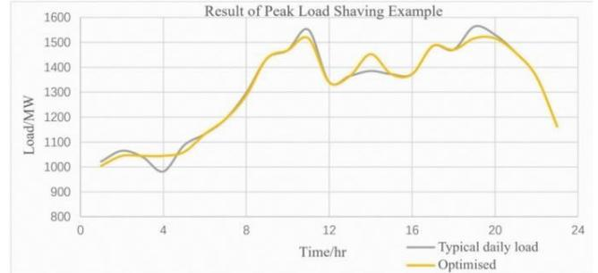
Figure 2: EV aggregation charging/discharging result
