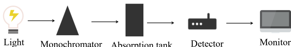
Figure 1: Basic structure of spectrophotometer
