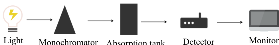
Figure 1: Basic structure of spectrophotometer
