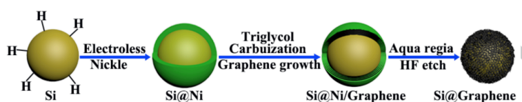
Figure 1. The synthesis process to obtain Si-C [9]
