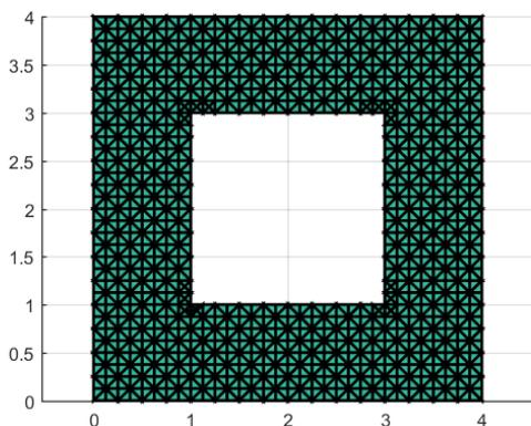
Figure 1: Adaptive mesh refinement 2 times
