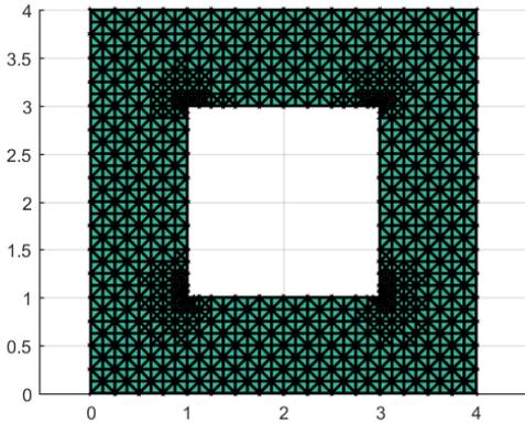
Figure 3: Adaptive mesh refinement 4 times
