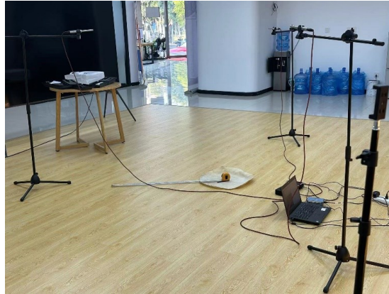
Figure 15: Experimental configuration for the sound evaluation of the violin bow subject to different pretension
