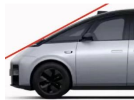
Figure 5: Angle between front windshield and the front cover of mega
