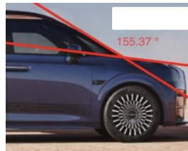
Figure 4: Angle between front windshield and the front cover of 009
