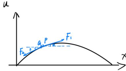
Figure 2: The Physical Model of String Vibration
