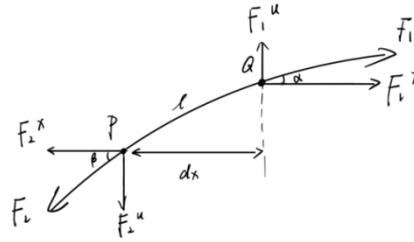
Figure 3: The Mathematical Model of String Vibration
