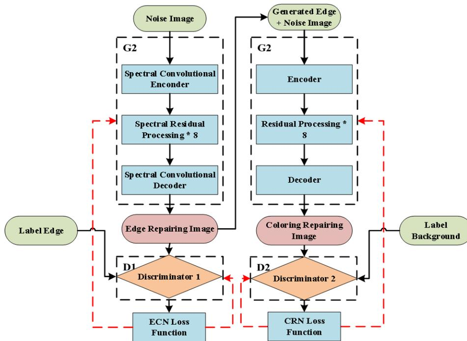
**Figure 1.** Proposed SHEN model. All noise images (Stream X) and Non-noise images (stream Y) from the selected training databases. The ECN network structure consists of G1 and D1. The CRN network structure consists of G2 and D2.
