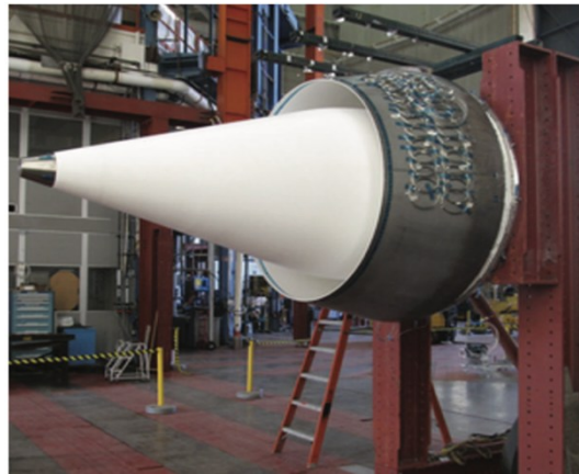
Figure 1: Oxide ceramic matrix composites exhaust ground test demonstrator consisting of a 1.60m diameter nozzle (showing underneath the titanium-alloy faring) and 1.14m diameter by 2.34 m conical center body with titanium end cap inspection portal (Courtesy of Wiley, Steyer [7])
