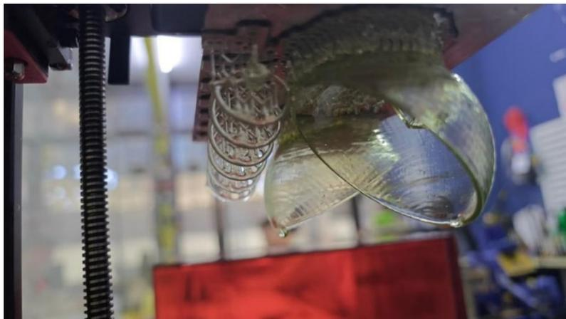
Figure 1: The model shell printed with light-curing 3D printing technology
