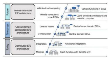
Figure 1: Centralized vs. distributed architectures [7]
