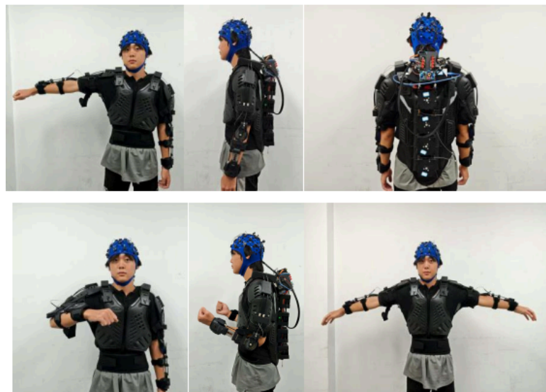
Figure 20. Range of arm postures demonstrating alignment and support of the finalized upper limb exoskeleton
